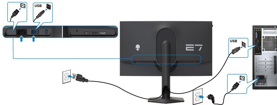
Figure 26. Connecting the USB cable
