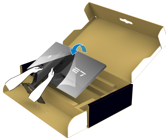
Figure 17. Hold the stand riser and lift the monitor.
