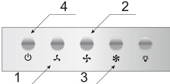
The control panel is equipped with buttons (isostat switch). To turn on the kitchen hood, press one of the button to select the desired speed:
